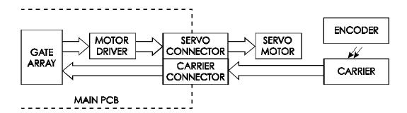
Figure 2-7. Servo Motor Controller.
